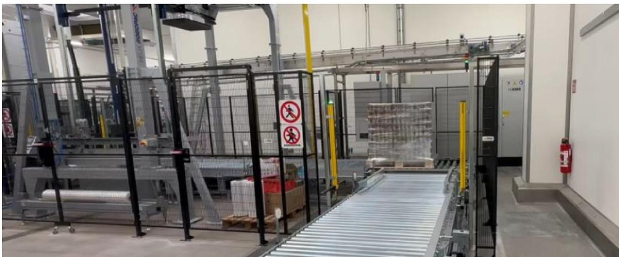
**Pallet wrapping / stretching / labelling of the finished pallet**
