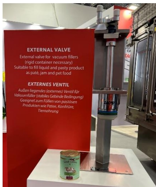
Example of an „external“ filling valve for vacuum fillers.
